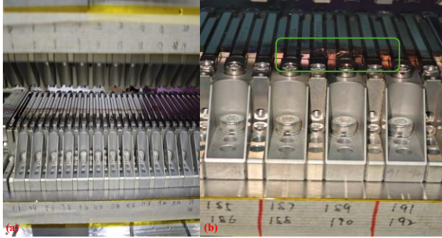
Figure 3: Damage to magnet blocks and poles: (a) surface charring; (b) pitting.
