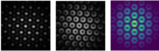
Figure 5: Reference and simulated far-field interference patterns used for mode discrimination. Left: Gaussian-like beam with l = 0 , showing a circular bright-spot array. Middle: vortex beam with l = -1 , showing a hexagonal-like pattern [14]. Right: multipinhole far-field interference pattern calculated from the GENESIS output field in the present work.
