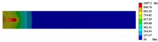
Figure 8: Two-dimensional temperature map on the foil for future high-power operation of the 1.5-MW MLF.
