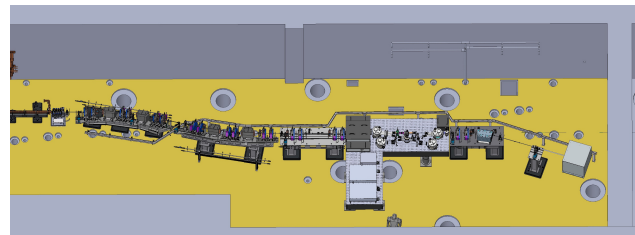
Figure 3: The transport line and the interaction section of the ELI-NP GBS.
