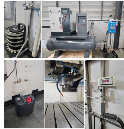
Figure 3: Ethanol spray cooling system installed at N.K.R. Engineering Company for oil-free five-axis CNC machining of the VCB-4 chamber halves.
