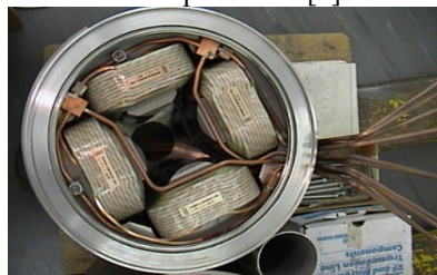
Figure 1: A quadrupole magnet with copper coil made of small diameter tubes with narrow elbows, filled with distilled water at a low flow rate (to counteract erosion).
