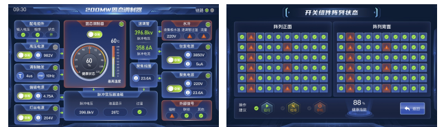
Figure 3: Control and health-management interface of the modulator, showing real-time module status, fault location, and the calculated health index of the module array.
