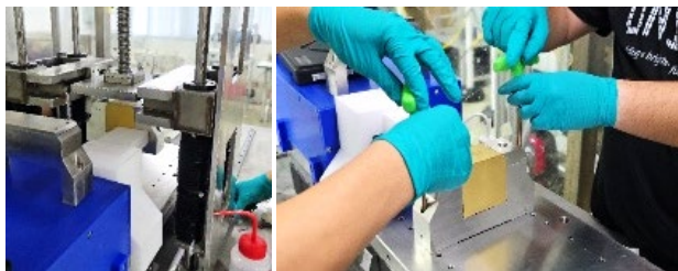
Figure 4: Mechanical integration of magnet blocks onto the girder utilizing a custom lead screw assembly system.
