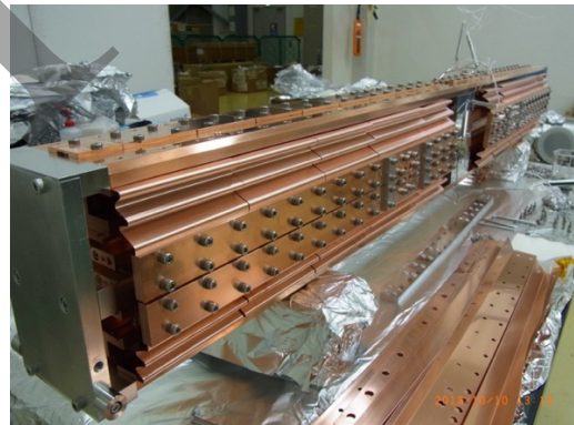
Figure 2: Copper plate and strips connected to in-vacuum girders of the CPMU15 at SPring-8.
