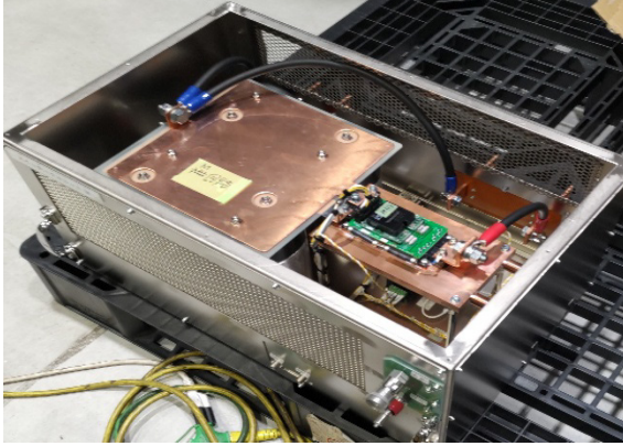
Figure 4: Photograph of test unit using SiC module.
