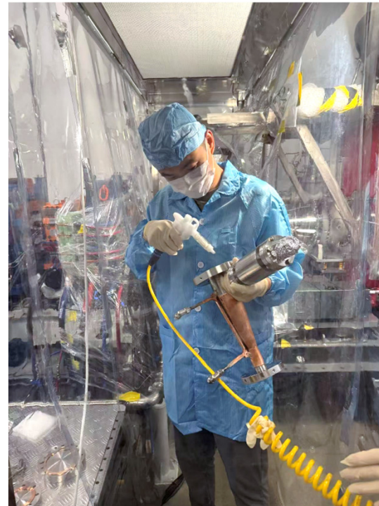
Purge w/ dust-free nitrogen
