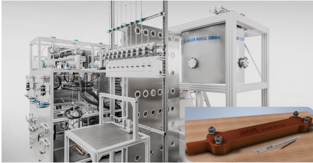
Figure 4: COMPASS teststand and worlds first operational prototype for 10 kA CMRC current lead.
