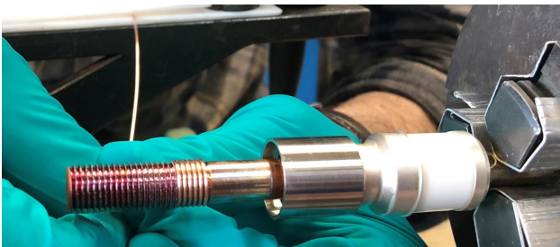
Figure 9: LTS wiring on specific machined feedthrough.
