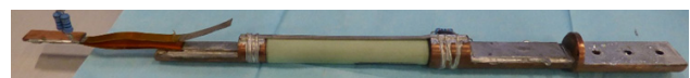
Figure 2: HTS lead assembly. YBCO tapes on the left, Bi-SCCO rod on the right.
