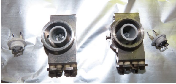
Figure 2: Sb and Cs crucibles with their heating filament.
