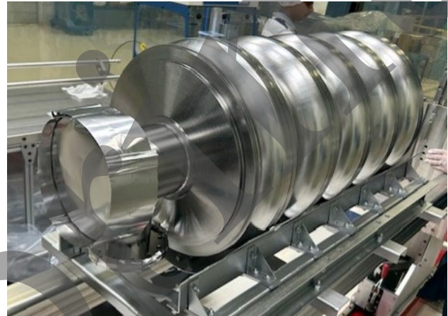
Figure 2: Cavity #401 Ready to Receive Mid-T Baking at Fermilab.
