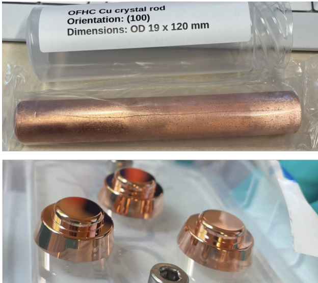
Figure 2: Substrate Cu(100) rod and three cathode heads produced for a cathode plug for the REGAE S-band gun.
