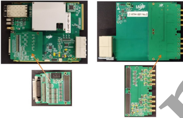
Figure 3: Tuning control board including AMC and RTM modules.
