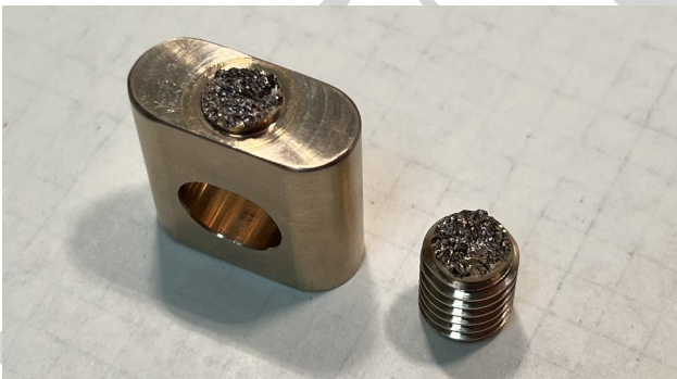
Figure 2: Failed jaw connection clevis adapter. Note the brittle appearance of the metal at the failure point.
