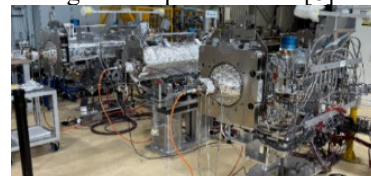
Figure 2: Three pre-series collimators at CERN.
