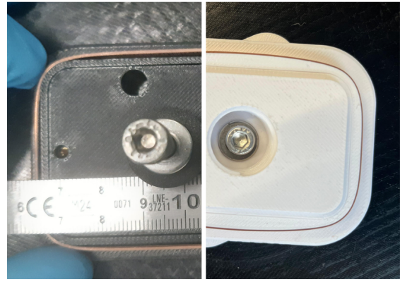
Figure 3: Tape tensioning test. Left: initial filleted rectangle mandrel. Right: optimized multi-arc mandrel geometry with improved contact and reduced stress concentrations.
