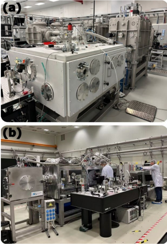
Figure 1: The kHz LWFA beamlines available at ELI ERIC: (a) The ELI-Beamlines ALFA based on L1-Allegro laser and (b) the ELI-ALPS eSYLOS based on SYLOS lasers.
