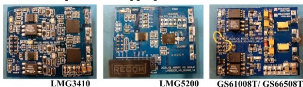
Figure 3: Homemade GaN FET power module.
