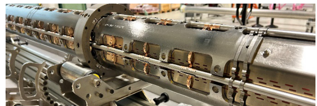
Figure 5: Beam screen with the Q2 shielding assembly.
