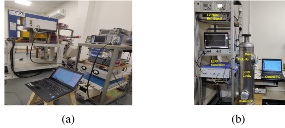
Figure 5: Test setup of TT Cyclotron (a) and SCRF Cavity at room-temperature (b).
