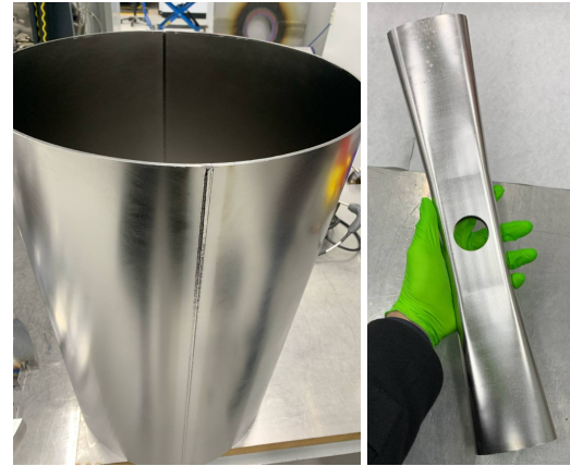
Figure 2: CST model of CH3 cavity (upper picture). Manufactured parts of cavity CH3. Left lower: Welded two-arched main cylindrical body immediately after welding (welding seam visible between arches). Right lower: One of the CH cavity spokes.
