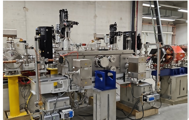
Figure 1: The STERN experimental chamber installed in the EuXFEL tunnel.
