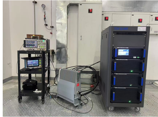
Figure 2: Photograph of the amplifier test bench and the assembled power amplifier unit.
