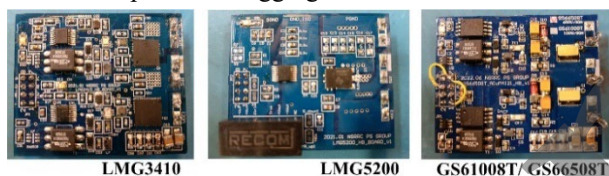
Figure 3: Homemade GaN FET power module.
