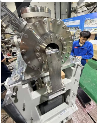
Figure 7: A mirror chamber of the resonant cavity.
