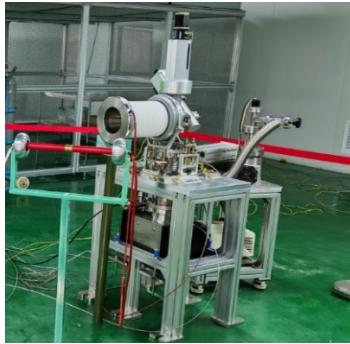
Figure 3: The electron gun undergoing high voltage test.
