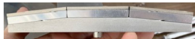
Figure 5: Three 50×50 mm magnet plates are arranged at a 5-degree angle to prevent neutrons from suddenly encountering the edges of the magnets.
