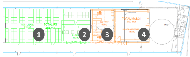
Figure 6: Laboratories and storage area in Prisma building. Four spaces are reserved for: (1) PS racks storage, (2) PS tests, (3) MA measurements and (4) GI and MA assembly area.
