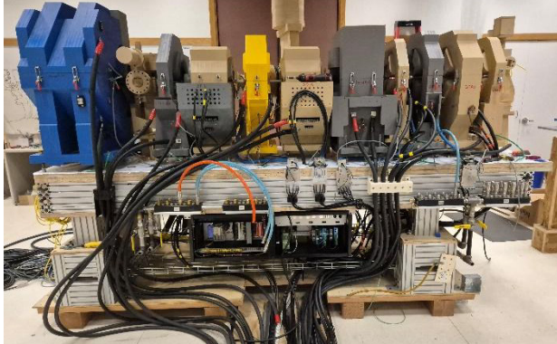
Figure 2: SR module mockup with mockup cabling in progress.
