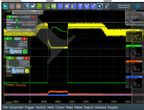
Figure 7: Phase probe (yellow) and FDC signal (green) of the 1.9 MeV beam behind the RFQ-IH-DTL from measurements on 3 March 2026 with a peak current of 6 mA.
