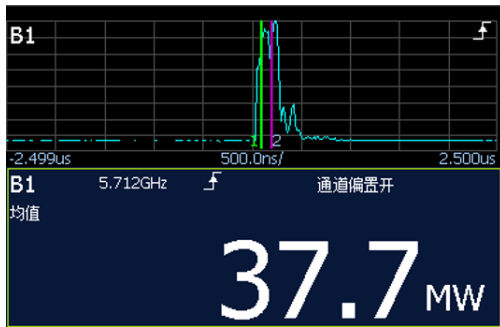
Figure 6: Output pulse waveform at the maximum power level.
