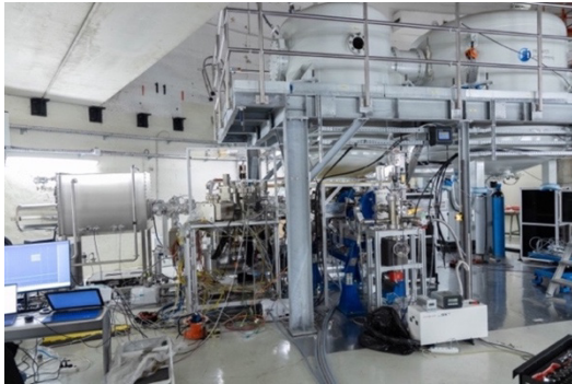
Figure 4: Photograph of the electron gun, below the HV platform and tanks, connected to the photocathode preparation facility (left) and to a short beamline (blue frame) ended with a Faraday cup (not yet shielded).
