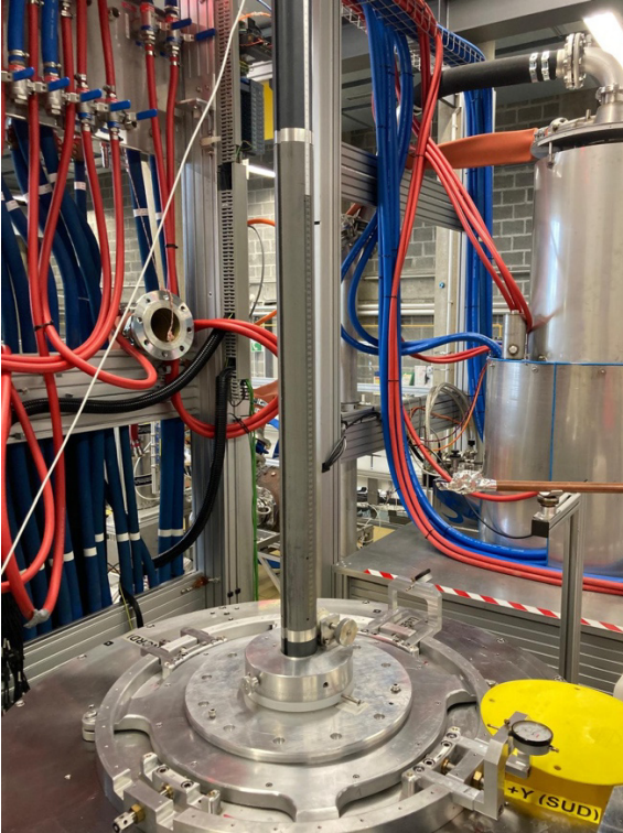
Figure 4: Custom-made probe holder for the SENIS 3MH6-E probe.
