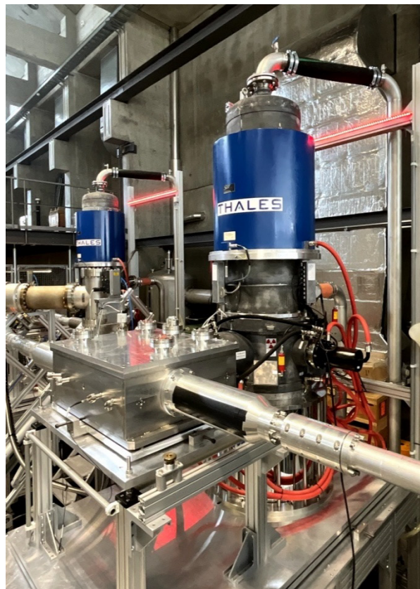
Figure 3: Two high-power gyrotrons used for plasma heating at the Swiss Plasma Center (SPC).
