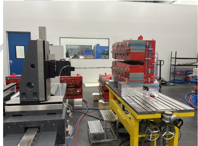
Figure 4: Hall probe measurement system for measuring LGB magnet.
