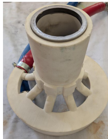
Figure 2: Glass-filled nylon cooling jacket assembled over the plasma chamber.
