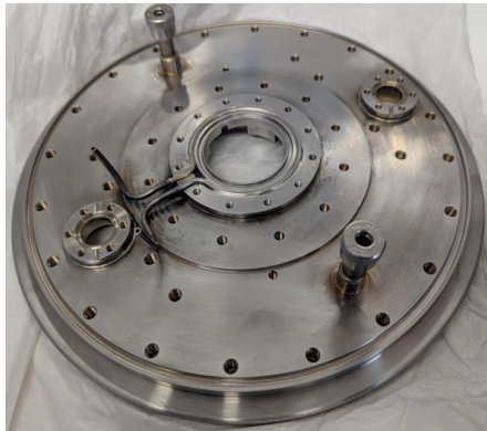
Figure 6: Main flange — machined and brazed.
