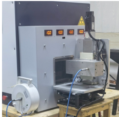
Figure 3: Focal spot measured by slit scanning method.
