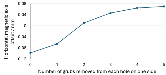
Figure 6: Simulation of correction of magnetic axis position arising from a 50 \mu\text{m} offset of one half of the outer yoke.
