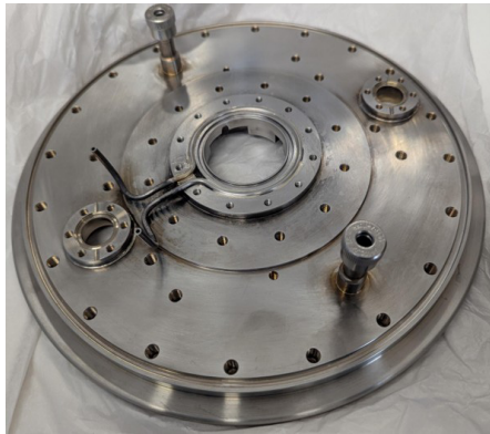
Figure 6: Main flange — machined and brazed.
