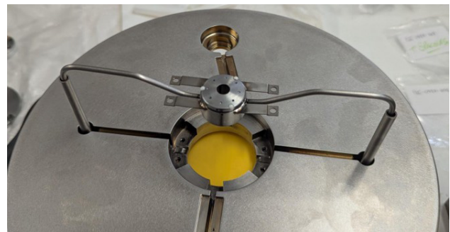
Figure 4: Caesium delivery system during assembly.
