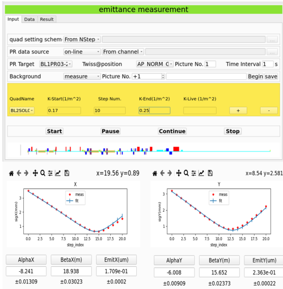
Figure 3: Emittance measurement GUI with solenoid-scanning option (Up), and the corresponding result based on virtual accelerator (Down).
