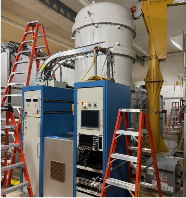
Figure 3: The assembled DTI power supply operated at 600 kV.
