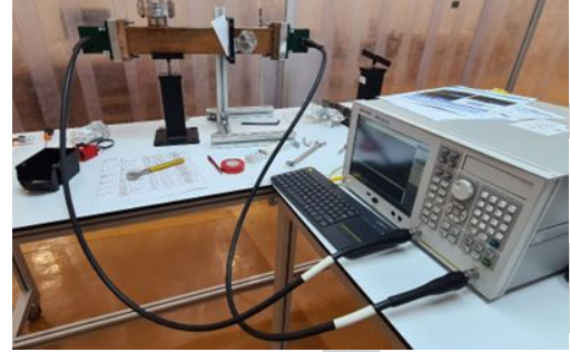
Figure 8: Setup for measurement of S-parameters of directional couplers.
