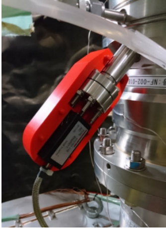
Figure 3: PM secured with a 3D printed holder in front of a viewport, monitoring the vacuum side of the window of a power coupler.
