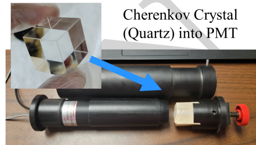
Figure 2: A quartz Cherenkov radiator with PMT assembly used in the Upstream Extinction Monitor.
