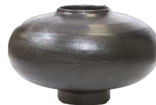
Figure 2: lateral view of the 1.3 GHz stainless steel cavity prototype
