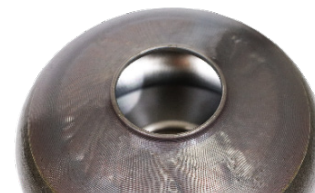
Figure 3: top view of the 1.3 GHz stainless steel cavity prototype after the final CNC machining
