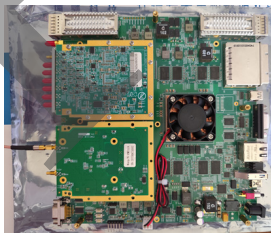
Figure 4: Customized beam current signal processor equipped with a high-speed (1 GHz sampling rate) ADC and a high-precision (24-bits) ADC.
