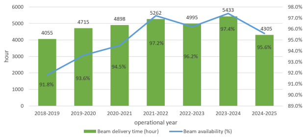
Figure 3: Delivered Beam Time and Beam Availability by Operational Year.
